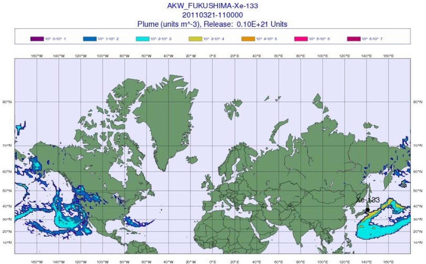
Figure: Simulated Radioxenon concentrations (Xenon-133) close to the surface (0-30 m).
