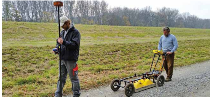
Bodenuntersuchung mittels Georadar entlang eines Damms Examination of the ground along a barrier by Georadar
