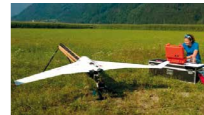
Die Messdrohne am Startkatapult The measurement drone in its start catapult
